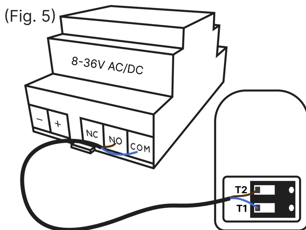
Polarity does not matter for most systems — the relay acts like a switch closing or opening the circuit. Turn your system back on. The relay's LED will blink if powered.
