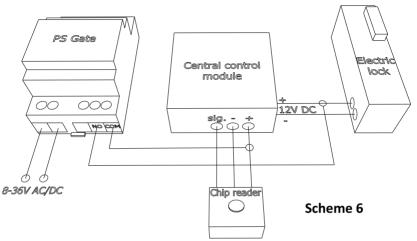
2.2 **PS Gate** is parallelly connected to the central control module **(Scheme 6)** and sends direct charge through the **NO** contact to the lock + 12V DC. This type of connection is allowed if the electric lock uses a direct current and its supply voltage is the same as the central control module one. Supply voltage could be sent to the central control module's exit. **PS Gate** could be used for control of central control modules with relayed exit.
