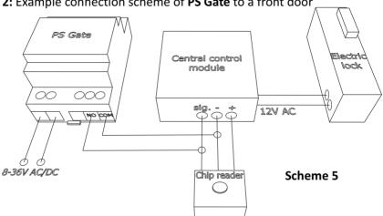
Step 2: Example connection scheme of PS Gate to a front door
