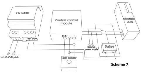
2.3 **PS Gate** controls external relay through an **NO** contact **(Scheme 7)** which is powered by the central control module's power supply.
